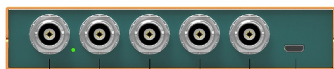
SDI out 9 SDI out 8 SDI out 7 SDI out 6 SDI out 5 Micro USB
